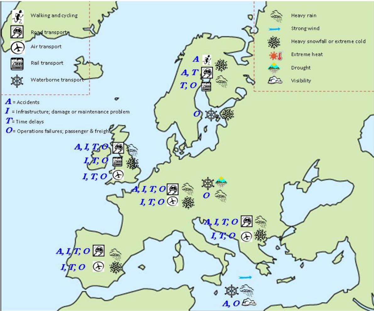
**Figure 2. Sum-up of critical weather phenomena, their occurrence by region where effects are the most severe, with the most affected modes of transport and the consequences (1)**
