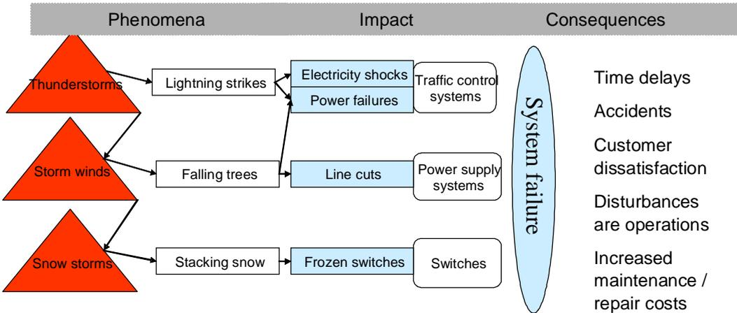
**Figure 1. Simplified impacts and consequences of harmful weather in rail transport (1)**
